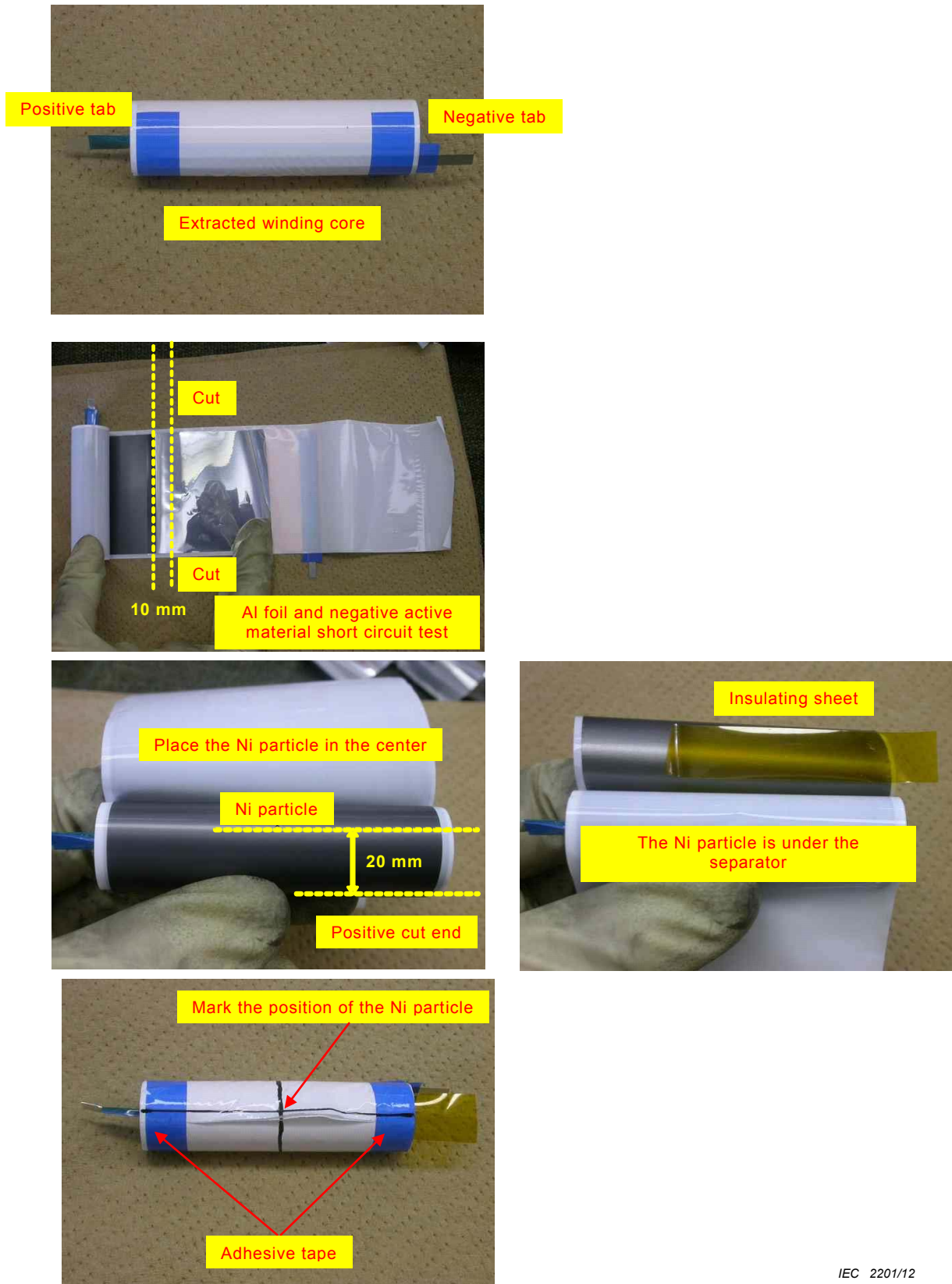
Figure A.5 – Disassembly of cylindrical cell
